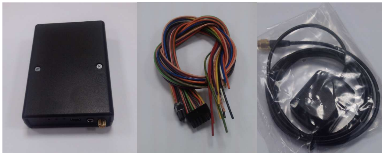
Figure2. FM-Eco3 device, power and I/O cables and GPS/GLONASS antenna.
